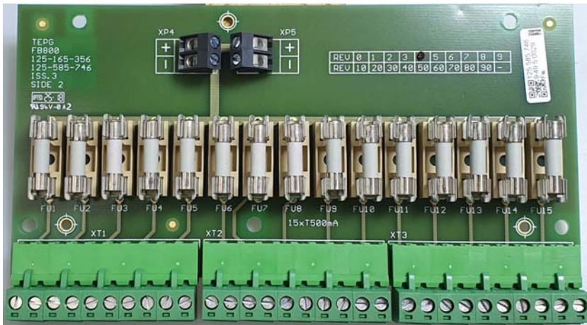
Fig. 1: FB800 Spare Fuse Board
