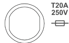
Illustration 22: Emergency power fuse
