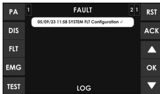
Illustration 44: Failure state log window
