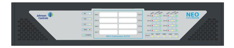
LDA NEO Extension 8250 is an extension unit for the EN 54–16 PA/VA system NEO. This extension unit scales the NEO system with 8 more zones as it includes 8 class D power amplifier channels of 250W at 100V or 70V.
