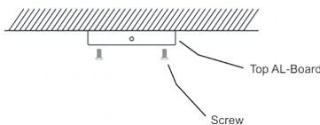
3. Align and slide the loudspeaker to the aluminium mounting piece and then tighten screws with the hex wrench.
