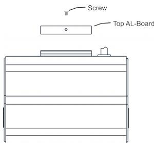
2. Secure aluminium mounting piece to ceiling or wall with screws.
