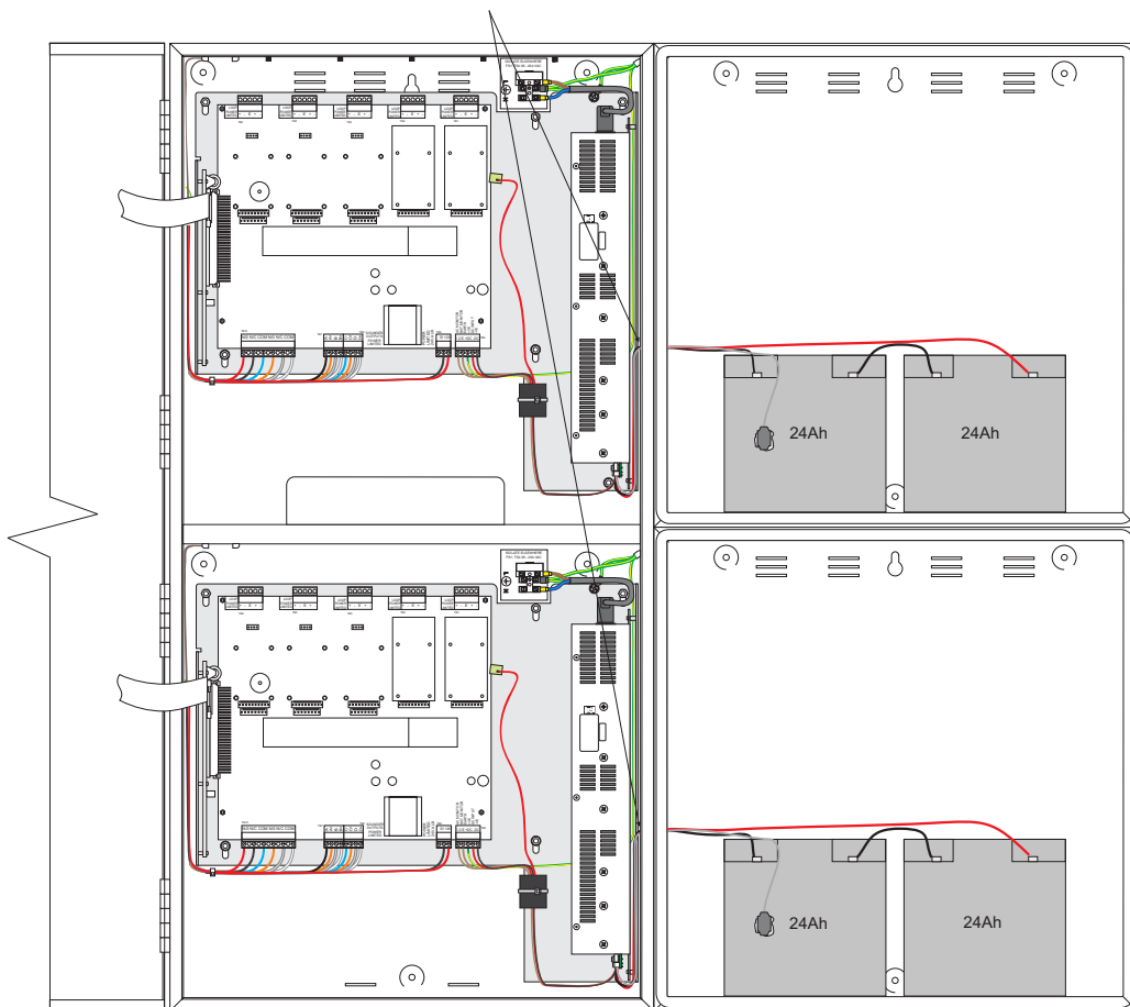
Figure 36 – ZX10Se Battery Installation – 17Ah or Greater
