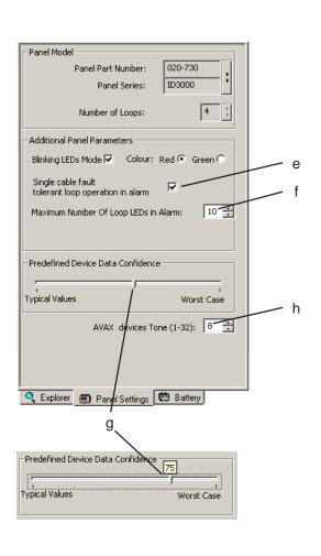
changed to green. Green LEDs use more current than red LEDs (red LED = 3.5mA, green LED = 7mA).
