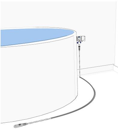
3. Attach the bracket to the wall with three screws. Recommended screw size is Philips #6 x 1 in. long.
