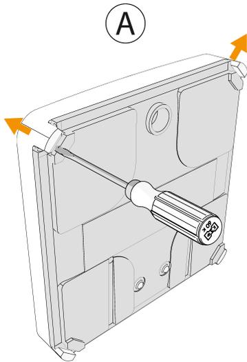
ⓘ **Note:** Do not use an electric screwdriver. This causes damage to the plastic enclosure.
