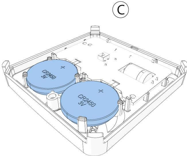
4. Pull the front clasp back and release the battery. See [Figure 3](#).
