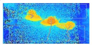
Avoid direct point light to ToF sensor, which may result in incorrect counting.
