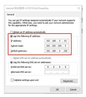
Step 3: Open the Browser and type 192.168.5.220 to access the web GUI. After logging on web GUI successfully, user is allowed to view configuration page.
