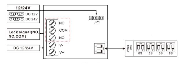
Note: A time delay is only supported for model ML5002LT
