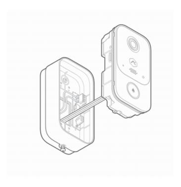
10. Fasten the security screw at the bottom of the wall mount assembly.
